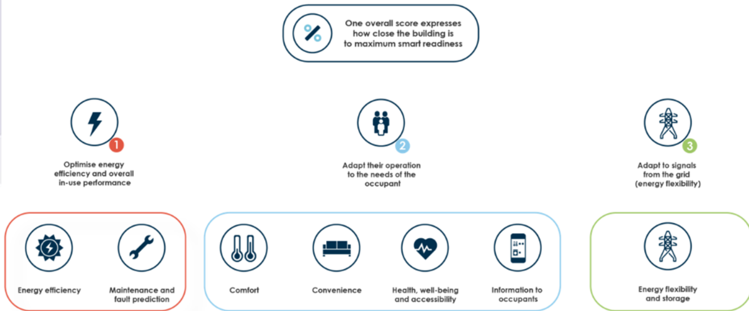
Figure 2 – Three key functionalities of smart readiness in buildings
